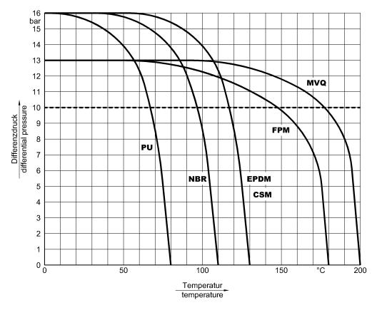
From DN 200 the use of seats with higher shore hardness is necessary at a differential pressure of more than 13 bar. Lug type valves:
