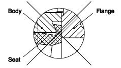
Remove the flange-spreaders and tighten the flange screws slightly and evenly <u>crosswise</u> with <u>the disc fully opened</u>.
