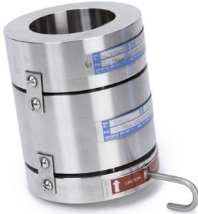
A Double Disc Holder Assembly consists of three holder components: an inlet, a mid-flange and an outlet piece, along with two rupture discs. The first of the two rupture discs is located between the inlet and the mid-flange, and the second rupture disc is between the mid-flange and outlet.
