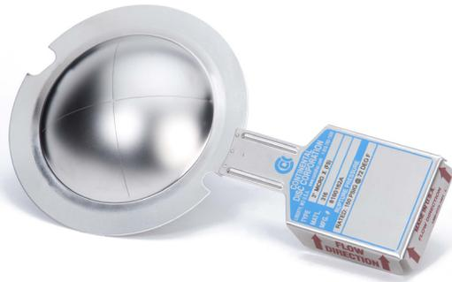
The **MICRO X® Rupture Disc** is a cross-scored flat seat tension type rupture disc. It is designed for non-fragmentation with a four-petal opening.
