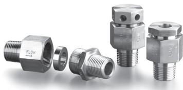
The **Tite-Seal Rupture Disc Assembly** is an economical "throwaway" sealed unit available with 1/4", 3/8", 1/2", 3/4" or 1" MNPT inlet connections and outlet configurations with an MNPT connection, muffled or free vent.
