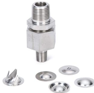
Screw Type Holders are available for pressures ranging up to 15,000 psig. The Screw Type holder is supplied with 1/4" or 1/2" MNPT inlet threads in combination with MNPT free or muffled outlets. The 1/2" Standard and 11/16" Composite Rupture Disc are used in these holders. Special high pressure designs are available.
