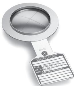
The **ICON Rupture Disc** is a cross-scored, non-fragmenting design solid metal rupture disc specifically designed to protect transportation vessels like intermodal tank containers (common in Europe and Asia), railroad tank cars, tank trucks, and other vessels that transport liquids or gas products.
