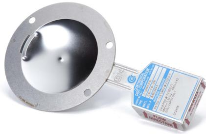
The **LOTRX® Rupture Disc** is a scored reverse acting rupture disc that utilizes failure initiating indents, a highly accurate manufacturing method to achieve and control a burst pressure at close tolerances, plus a precision semicircular score to provide a clean, consistent opening pattern.
