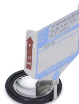
The **SANITRX HPX® II Rupture Disc** is designed to expand the SANITRX HPX® product line into higher burst pressure ratings. The geometrically strengthened arcuate on the SANITRX HPX® II provides a radiused hinge point to prevent fragmentation of the rupture disc petal upon rupture. SANITRX HPX® II also adds the 4" size rupture disc to the SANITRX HPX® Rupture Disc product family.
