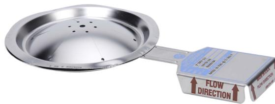
The **Composite Rupture Disc** is designed for systems requiring a lower burst pressure than offered in Standard discs. Continental Disc Corporation's seven-hole center pattern is designed for non-fragmentation when used with a TEFLON® seal.
