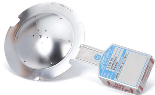
The **Composite Flat Seat Rupture Disc** is designed for systems requiring a lower burst pressure than offered in a MICRO X® Rupture Disc. Continental Disc Corporation's seven-hole center pattern provides a non-fragmenting design when used with a TEFLON® seal.
