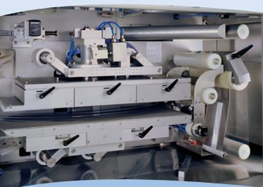
Forming station and index with integrated cooling
