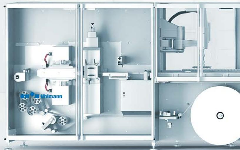
BLU 400 with SyPro feeder, sealing and punching station, plus C 2305
