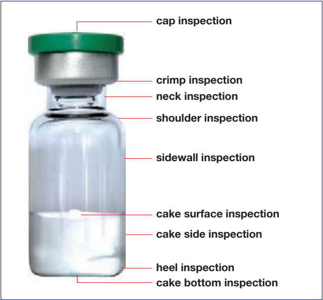
Typical inspection criteria of vials filled with lyophilized product
