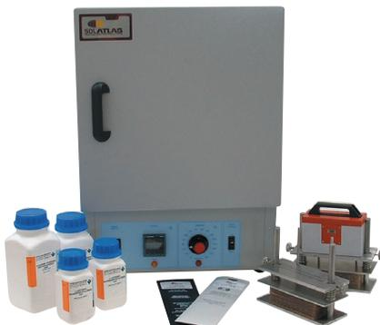
To determine colorfastness to water and perspiration of textiles. Provided with 2 stainless steel frames each with a capacity of 20 samples of 10 cm x 4 cm held between acrylic separator plates. Loading weights for BS, ISO and AATCC standards are included. An electric incubator is required available but not included.
