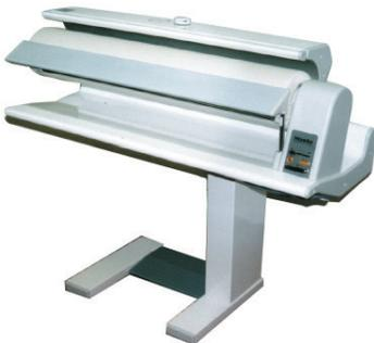
Conveniently determines the ironability of various fabrics. With certain modifications the Rotary Ironer is suitable for specific Marks and Spencer Plc test methods but in this form is restricted to accredited M&S suppliers.
