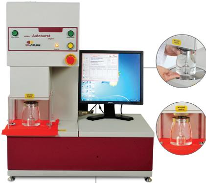
The Autoburst is a hydraulic bursting tester with advanced testing controls. The instrument has automatic flow control allowing bursts to be achieved within the specified time of the standard. The advanced software provides diaphragm correction calculations for consistent results. These features, along with a maximum capacity of 6000 kPa (871 psi), make the Autoburst the most versatile burst tester on the market.
