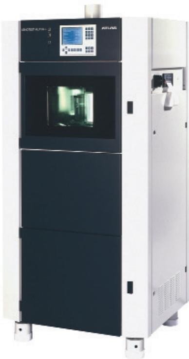
A compact, state-of-the-art design. Xenotest Alpha is the universal weathering instrument for testing the lightfastness and weatherability of materials under normal, high temperature and High Energy conditions.
