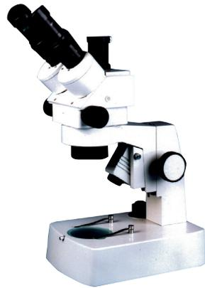
45° binocular stereo microscope with Greenough zoom optical system. Widefield eyepieces 10x, 0.75x-4.5x magnified range and 1.6 zoom ratio. Compact R2GG stand with halogen incident and transmitted light.
