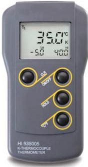
For accurate measurement of superheated surfaces, gases and liquids. With Thermocouple K-Type roller surface probe and general purpose probe (liquids and gases) - 50°C to 199.9°C and 200 to 1350°C, with accuracy  $\pm 0.2^\circ\text{C}$ . Battery operated with 1600 hours of battery life, LCD display with max/min temperature memory, hold facility and switchable  $^\circ\text{C}/^\circ\text{F}$  readout.
