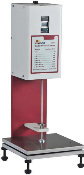
For carpet testing, with weight set 20-2000 GM/cm<sup>2</sup>, presser foot 412 mm<sup>2</sup>, range 0-25 mm x 0.01 mm.
