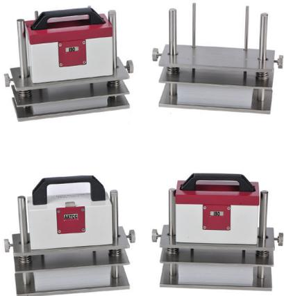
To determine the colorfastness to water and perspiration in textiles. A stainless steel frame with a capacity of 20 samples of 10 cm x 4 cm held between acrylic separator plates, loading weights not included. Comply with AATCC and ISO test methods by add on individual weights: 3.36 kg (8 lb) for AATCC, and additional weight 0.47 kg (1 lb) for ISO. An electric incubator is required.
