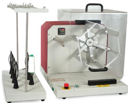
To produce skeins of yarn of a predetermined length and number of turns for count and/or strength testing, 1 Meter, 36" or 54" circumference collapsible swift (specify). Complete with yarn package stand and pretension device, fitted with predetermined counter. Available in hand operated and electronic versions.
