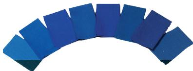
Blue wool fabric (pack of 8 graded 1-8) to meet ISO/SD/BS standards. Dimensions for each piece 240mm (9 1/2") x 150mm (6")
