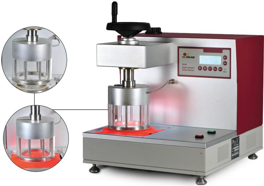
Powerful and intelligent, the HydroPro Hydrostatic Head Tester is designed to help labs be more efficient while meeting global standards. The compact design can reach 3 bar of pressure using standard lab compressed air. The quick-test function allows users to perform other tasks during the first 80% of the standard test. An alarm indicates fail pressure is close and a technician should begin observing. The test area is well lit behind a clear shield for observing when droplets appear.
