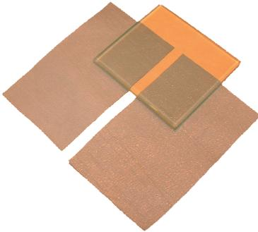
When a sample is observed to have lost color or have changed color during washing, this may be due to the effect of washing or the effect of the presence of optical brightener on the sample. This can be assessed using the fluorescence suppressor.
