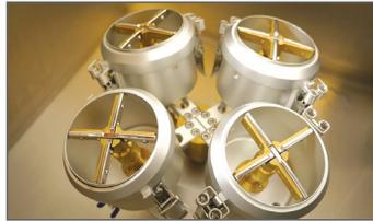
The Bundesmann provides a water repellency test for fabrics that are being contacted during use such as a rain jacket. Samples are mounted over a cup and are rubbed from underneath during the test. Three hundred precision stainless steel drop formers provide simulated rain falling from a height of 150 cm. Samples mount onto holders outside of the tester and then are easily set in place on top of the cups.
