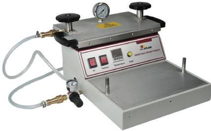
To distinguish between imperfections in fabric construction and streaking due to dyeing and finishing. By the controlled application of heat, pressure and cooling, a permanent impression of a test fabric is made from Optical quality polystyrene film, allowing objective analysis of external imperfections without the confusion of color or pattern.
