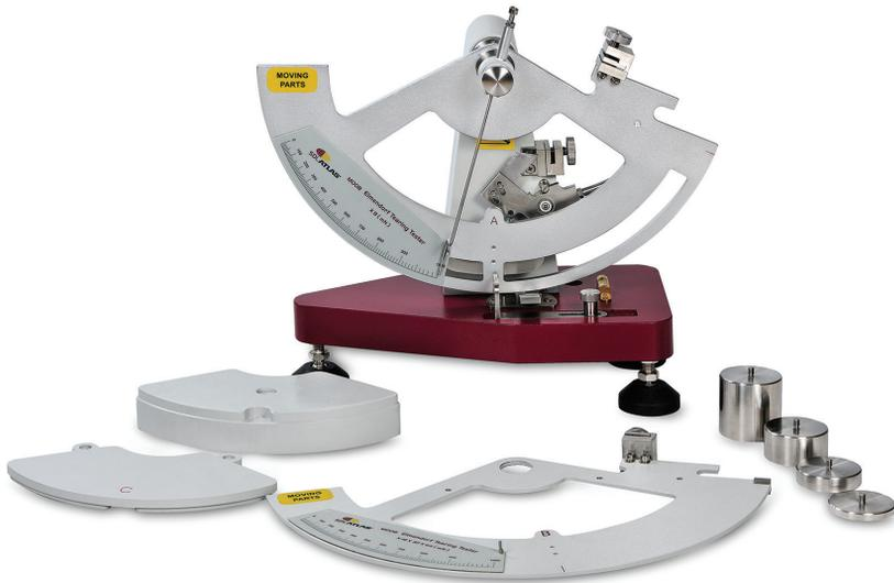
To determine the ballistic tearing strength of textiles, paper or board. Three interchangeable pendulums ranging from 8,000 to 64,000 Millinewtons (mN) can be selected separately for multiple test method compliance.
