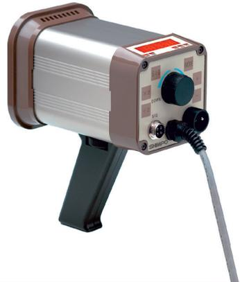
For taking non-contact RPM measurements and inspecting moving parts. Handheld with LCD display, NiMH battery, 1200 Lux flash at a distance of 20 cm to the object,  $\pm 0.01\%$  reading accuracy,  $\pm 1$ RPM resolution, Flash range 30 - 12500 FPM. May be externally triggered.
