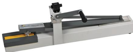
To determine the colorfastness of textiles to dry or wet rubbing. Motorized for frequent use and long run tests, fitted with digital electronic pre-settable counter for strokes up to 9999.
