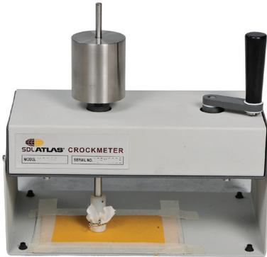
To determine the colorfastness of textiles to dry or wet rubbing particularly for printer fabrics. Applies 1134 grams of pressure on a 16 mm finger and rotates 1.125 turns clockwise then counter-clockwise. The operating handle is however turned in one direction only.
