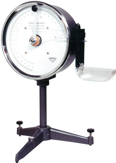
250° scale x 500 divisions. Ranges from 0-5 mg x 0.01 mg to 0-1000 mg x 2.0 mg. Also available scaled 0-500 denier for yarns (90 mm sample). Complete with pan, hook and draught excluder.
