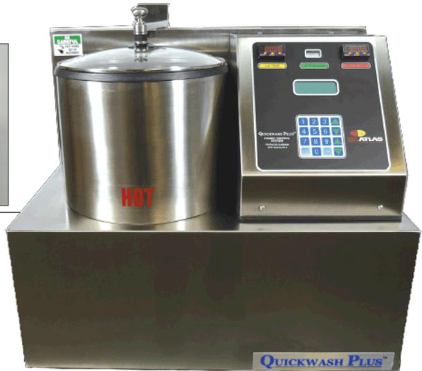
The QuickWash Plus gives fabric shrinkage information in a 12-15 minute test versus the 8-12 hours it takes a standard washer and dryer. This instrument is ideal for the factory floor and provides rapid, on the spot information on fabric in production so that the stenter frame, compactor, and sanforizer can be set to maximize fabric yield. This allows user to bypass the standard wash and dry cycles that take so long thus significantly reducing labor in the lab.
