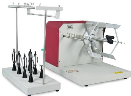
To produce skeins of yarn of a predetermined length and number of turns for count and/or strength testing, 1 meter, 36" or 54" circumference collapsible swift (specify). Complete with yarn package stand and pretension device, fitted with predetermined counter. Available in hand operated and electronic versions.
