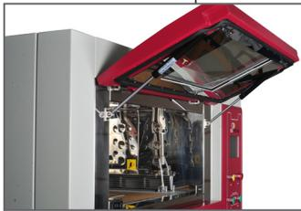
Often referred to as the “Skin Model”, the Sweating Guarded Hotplate (SGHP) measures thermal properties and water vapor resistance of fabrics and other materials under steady state conditions. The test simulates the heat and mass transfer process which occurs next to human skin.
