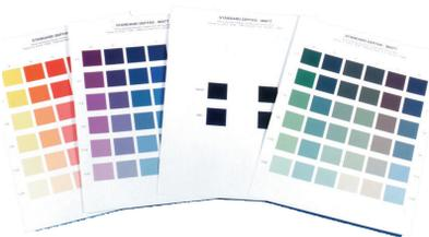
As the fastness of dyeing depends on the depth of color, it is necessary to specify standard depths when making comparisons. Dye manufacturers' pattern cards refer to these depths in fastness ratings for their products.
