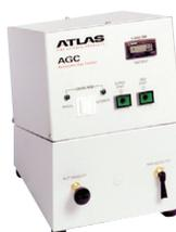
To determine the burning characteristics of textiles under controlled conditions. Stainless steel test cabinet with glass observation panel provided with automatic timing of flame spread in 0.1 second increments from ignition. Automatic or manual flame impingement for 1, 5 or 20 seconds. Brushing Device including Nylon Brush is available per request.
