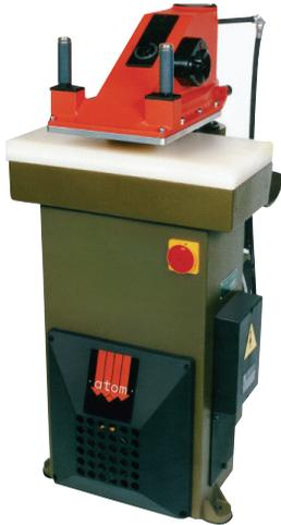
Swing arm cutting presses are ideally suited to cutting test samples from textiles, rubber and soft plastic prior to testing. Depending on resilience, several thicknesses can be cut at once with a cutting force of 20 tons. Control push buttons with time delay ensure complete operator safety. Maximum cutting area 18" (450mm) x 36" (900 mm). Cutting dies of any shape and size can be supplied.
