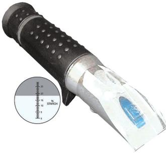
To determine the amount of starch or solids percentage in a sizing solution.
