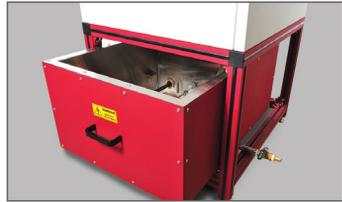
The Rain Tester provides a water repellency test for fabrics with different intensities of water impact at specified water temperature. Samples are mounted vertically while the simulated rain is sprayed horizontally. Samples are backed with a standard blotting paper that is weighed before and after the test. The Rain Tester provides precise control of the test through a color touch screen controller including water column height, water temperature, and test time.
