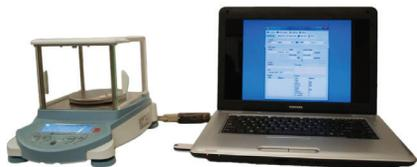
Consists of an electronic balance (220 grams x 0.001 grams) with internal and external custom software which calculates yarn, sliver and roving counts as well as fabric yield in various systems and provides statistics on any number of tests including totals, average, CV and SD. Includes cables and security data key, USB, and connects to any PC and printer. PC and Printer are not available.
