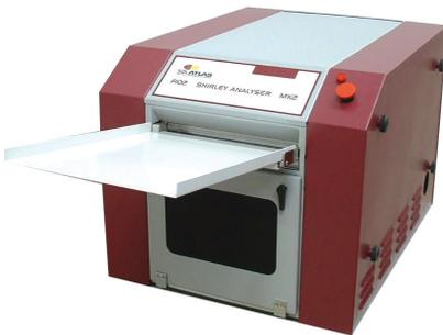
Lint and Trash Analyzer MK2 (Cotton Model). To determine lint, trash and dust content within a sample of cotton fiber up to 100 grams. Also used to determine non-fiber content of synthetic fibers and to open and clean fibers for further testing. The analyzer uses the carding principle with air separation of lint and non-lint content.
