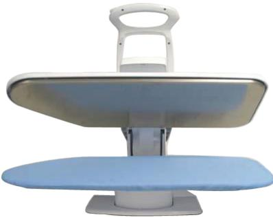
To determine the colorfastness of textiles of all kinds to domestic or industrial ironing. The instrument is formed by two parallel and smooth plates: the upper plate warms and exerts a pressure of 4 kPa on the specimen. The determination can be performed at different temperatures and in three ways:
