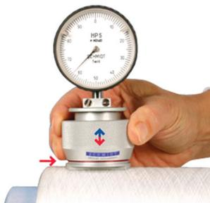
To measure the hardness of yarn cones or beams of yarn or fabric. Suitable for loosely wound bobbins of synthetic fibers and closely wound natural fibers, yarns and threads. Analog scale from 0-100 with 5 mm diameter indenter (supplied in fitted box).
