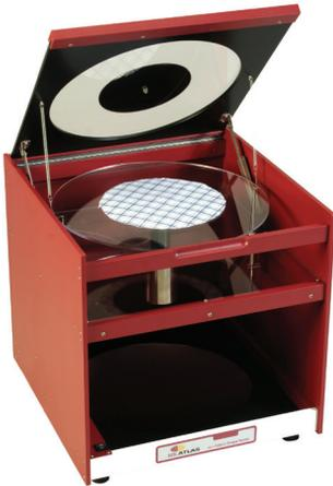
To measure and calculate the coefficient of drape by tracing a shadow of the draped fabric on paper. Supplied with three templates with paper rings with diameter of 24 cm, 30 cm and/ or 36 cm (50 pcs each).
