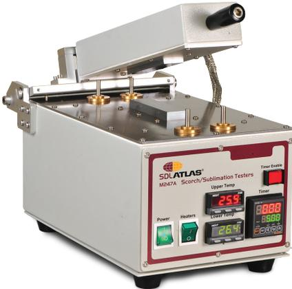
The Scorch Tester determines colorfastness and shrinkage to hot pressing and dry heat. This instrument is available in two different hot plate sizes. The top plate has a unique hinge and spring pin design to ensure even pressure across the sample. Each plate temperature is individually controlled and a timer is also integrated with the device.
