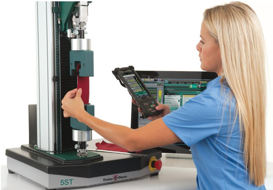
The ST series of electromechanical testing machines from Tinus Olsen are designed to test a wide range of materials in tensions, compression, flexure, shear, and peel.
