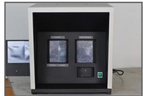
The ICI Mace Snag Tester is designed to test the snagging resistance of heavy duty fabrics used in apparel, upholstery, and automotive interiors. The instrument comes with a viewing assessment cabinet and standard photographs.
