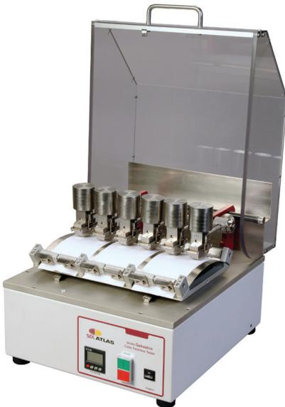
For evaluating a material's resistance to rubbing motion. Unit is a six station, benchtop machine which includes clamps for sample attachment to moving platen and clamps for weighted rubbing arm for attachment of rubbing material. Cycle counter automatically stops machine at end of test cycles. Test samples are visually evaluated.
