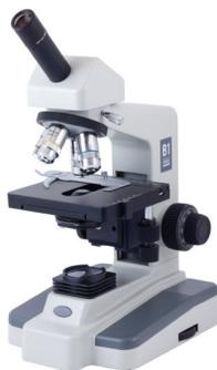
For the examination of textiles up to 1000 times magnification. Eye pieces 10x, objectives 4x, 10x, 40x and 100x, 12 V/20 W Halogen illumination with intensity adjustment, 45° inclined Monocular head with 360° rotatable head, coarse and fine focusing, vertical travel range 27 mm.
