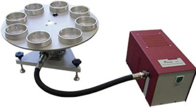
To determine the resistance of textiles and textile composites (particularly performance wear fabrics) to water vapor penetration. The apparatus consists of 8 containers with water reservoirs, a standard permeable fabric cover, sample holder ring and precision drive.
