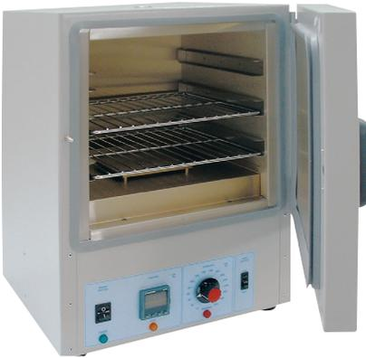
Dual purpose for both perspiration and oven-dry tests with high accuracy. 30 liter or 120 liter capacity. Dual temperature ranges and scales (25-110°C +/- 0.25°C, 50-250°C +/-0.75°C) stainless steel interior. Circulation fan and door thermometer, 2 shelves. Other sizes, temperature ranges and accuracies available upon request.
