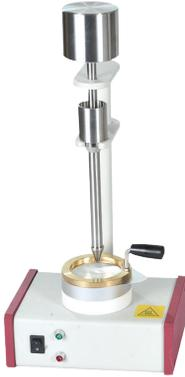
To determine the oil or finish content of wool or synthetic samples by solvent percolation and evaporation. Suitable for fiber, yarn or fabric. Available with 1, 2 or 3 extraction units. To be fully compliant with Edana method ERT 155, it needs a large extraction tube- 12 mm (OD), 10 mm (ID). (Full title of new method is: DETERMINATION OF ACETONE EXTRACTABLE FINISH ON NONWOVENS).
