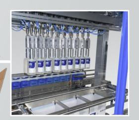
Flexible use of robots in the clean room for loading and unloading freeze dryers
