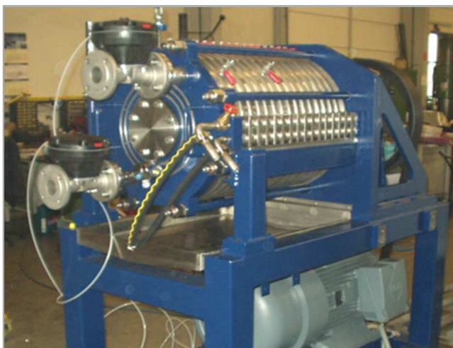
DYNO Filter in the workshop ( A_F = 6 \text{ m}^2 , 15 modules)
