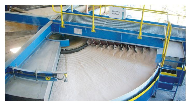
Pan filters with their horizontally arranged filter surface are particularly suited for filter cake washing. Therefore, they are preferably used for the filtration and washing of coarse-grained and rapidly sedimenting suspensions.
