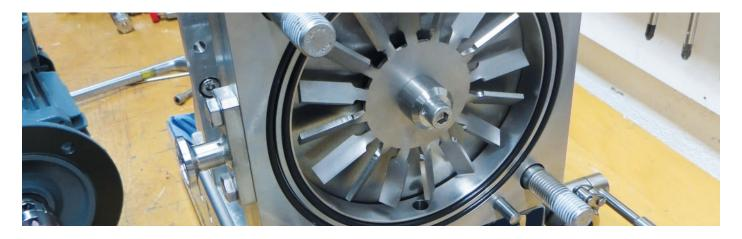
With small sample quantities, BoCrossTest enables the determination of the filtration behavior under crossflow conditions. Various suspensions and filter media (polymer membranes, metal mesh, ceramic membranes) can be investigated. BoCrossTest can be operated both, discontinuously and continuously.
