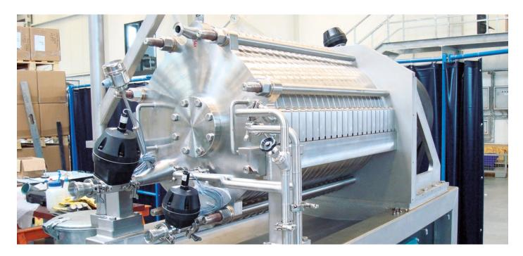
Dynamic crossflow filtration with the BoCross Dynamic filter is a unique process for microfiltration and ultrafiltration of microfine to nanoscale suspensions. Tasks such as thickening, washing and clarifying are performed by the BoCross Dynamic filter in continuous operation with permanently high throughput rates.
