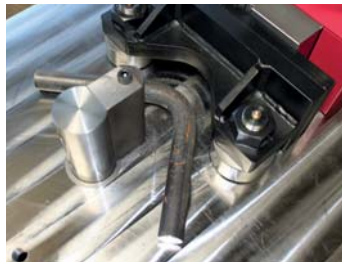
75 Rollenprisma Roller vee-block
