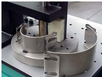
87 Blech > 90° biegen Bending of sheet metal > 90°
