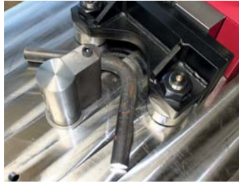
75 Rollenprisma Roller vee-block
