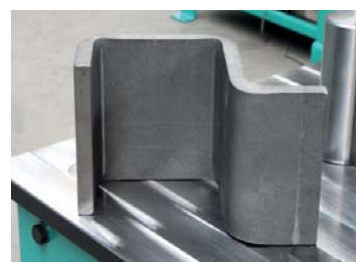
97 Dicker Flachstahl biegen Bending of thick flat steel
