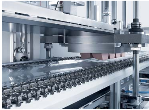
Blister forming station of the Blister Machine KBS-KF
