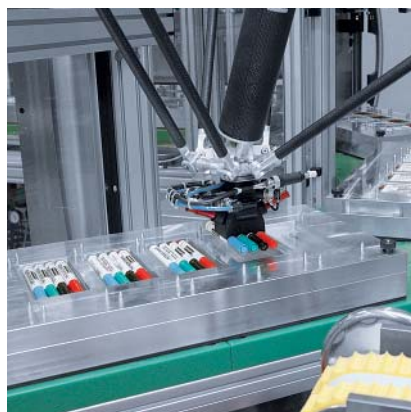
Pick-and-place handling ensures maximum servo-regulated precision
