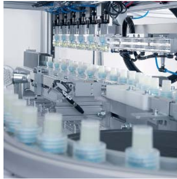
Feeding and handling system for a cosmetic product
