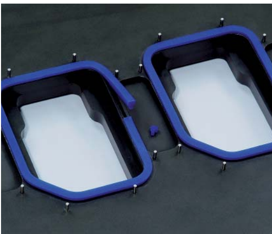
The rubber seals and spring pins on the sealing tools are easily replaced.
