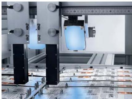
Example of a printing and camera system that marks and subsequently verifies variable product data
