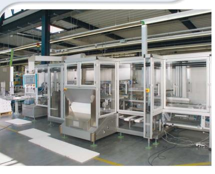
For years Höfliger has been one of the leading manufacturers of wallet packaging lines. As a rule the wallet packs are cartoned and packed into shipping cartons immediately after the production line.
